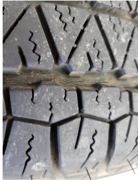
Splits and tears at the base of the treads.
