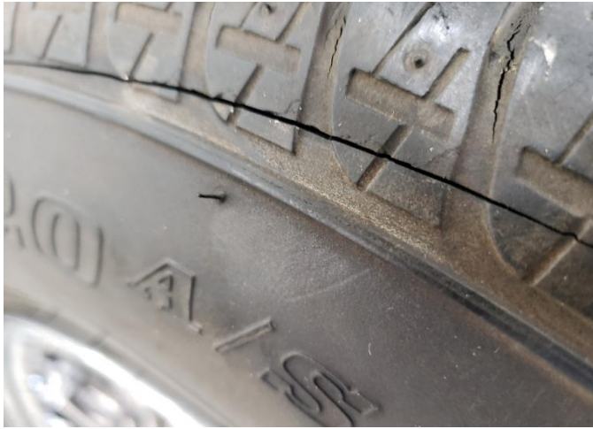
A tear across the tread and down the sidewall.
